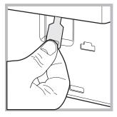
4. pull outwards using the tab as indicated in the figure, until the plastic tie-rod is freed from its stop position; pull downwards and open the door at the same time.
